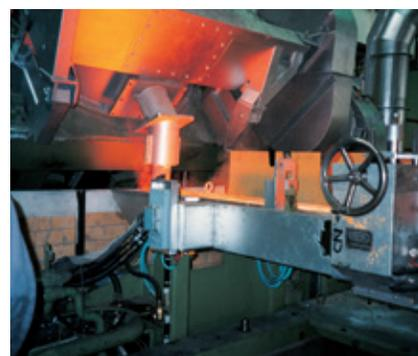
Furnace with pouring tube
