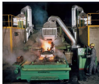
50-tonne MFT furnace serving a vertical continuous caster
