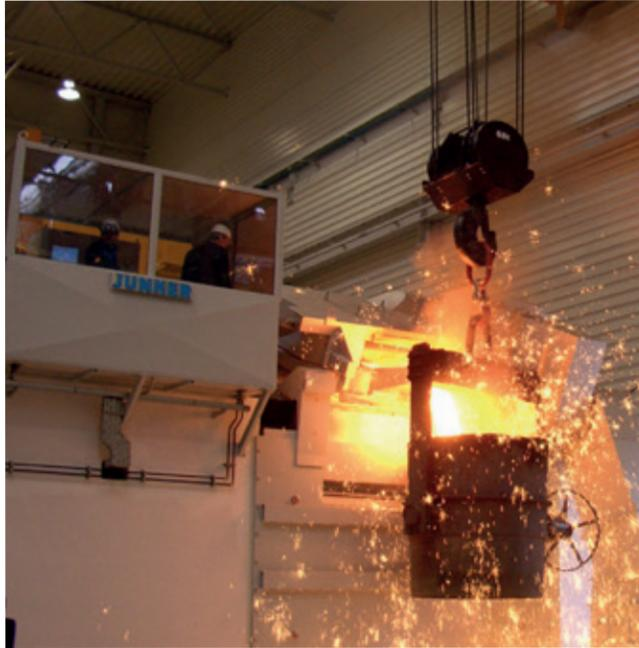
Powerful 9,000 kW cast iron melting furnace
