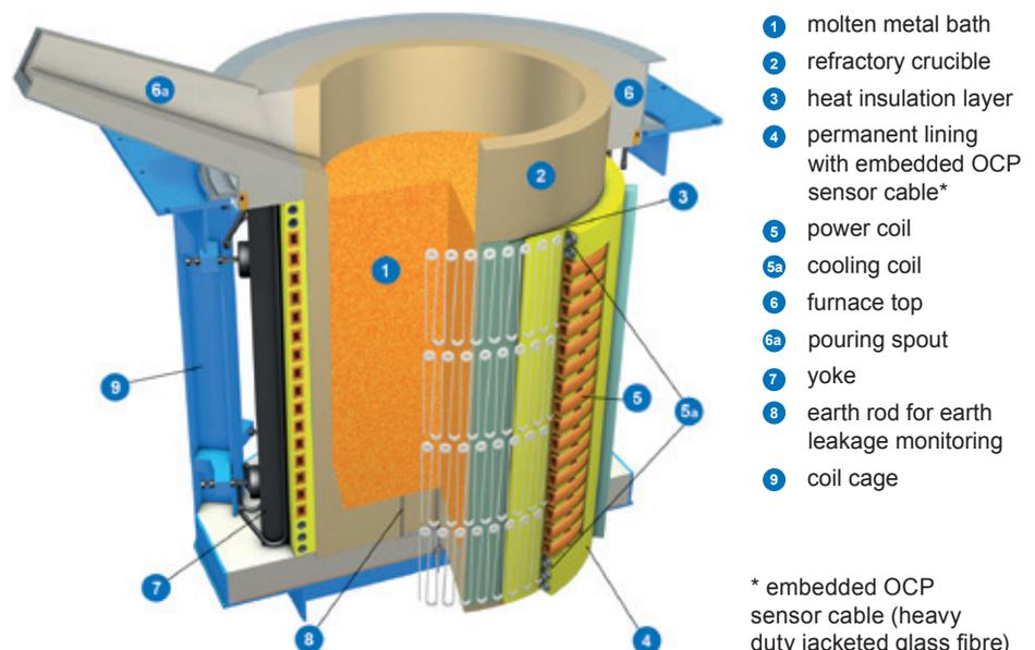
\* embedded OCP sensor cable (heavy duty jacketed glass fibre)
