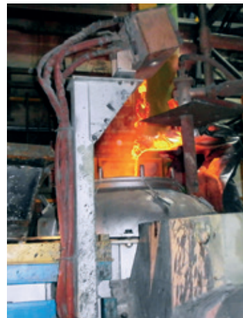
Pouring spout with float system and quickly replaceable stopper
